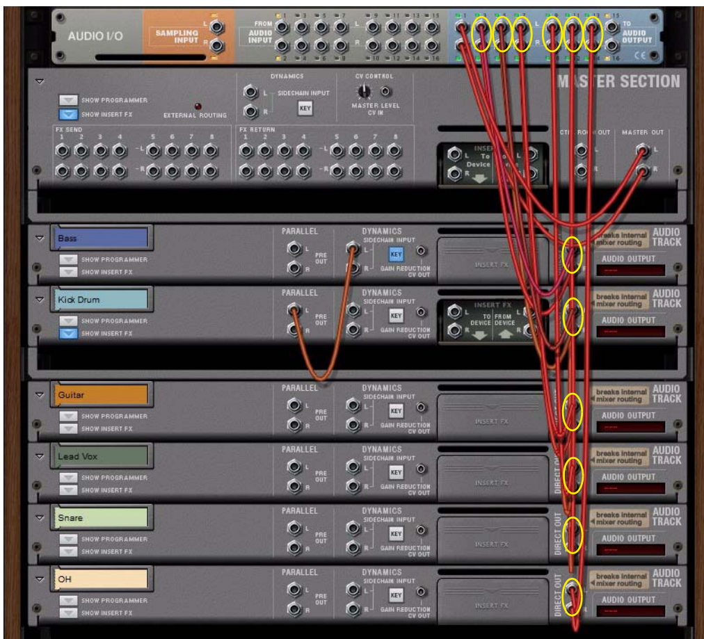
Direct routing of individual channel outputs to individual outputs on the Reason Hardware Interface
