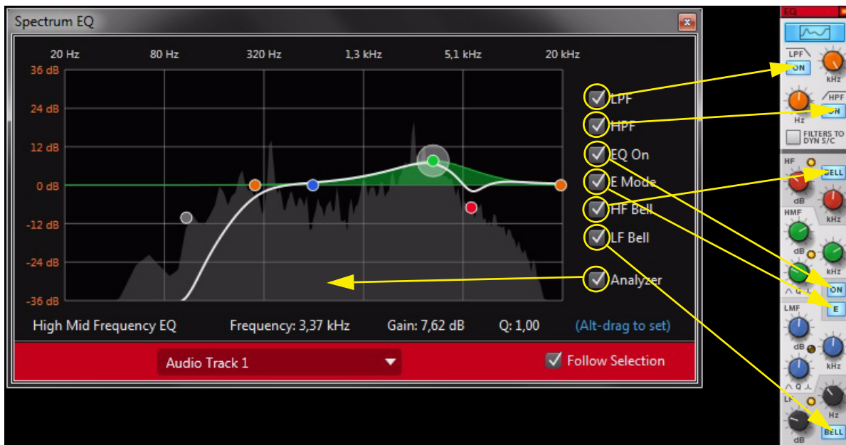
The Spectrum EQ Window with the Filters, EQ, E Mode, Bell Mode and Analyzer functions active during audio playback
