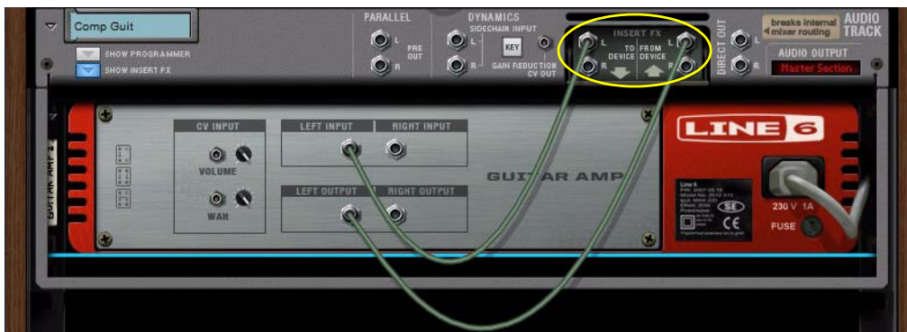
The "To Device" and "From Device" connections in the Insert FX slot in the Audio Track device
