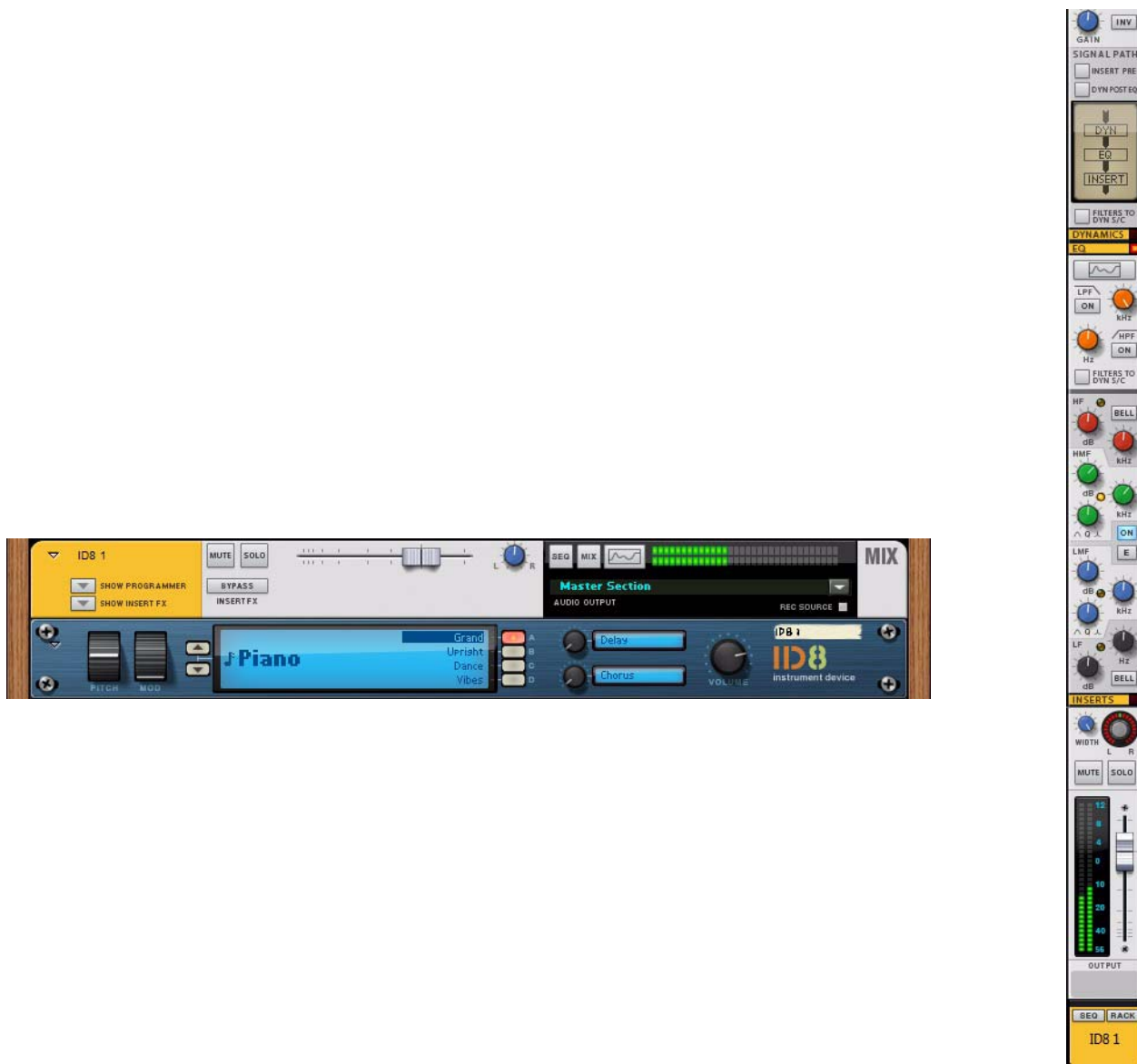
A Mix Channel device (with an ID8 source device connected) and the corresponding channel strip in the Main Mixer.
