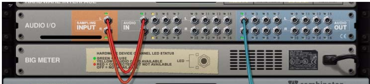
Audio Inputs 1&2 connected to Sampling Inputs L&R for sampling in stereo
