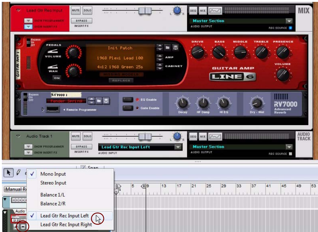
The Mix Channel device selected as audio input on the Audio Track in the sequencer
