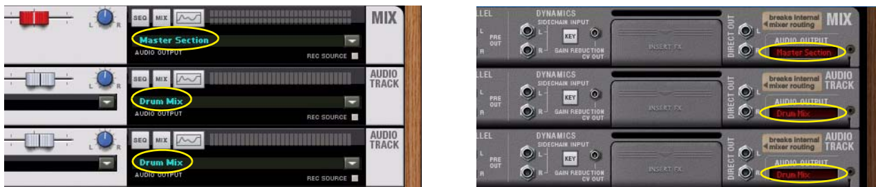
P-Lan signal destinations on Mix Channel and Audio Track devices (front and rear)
